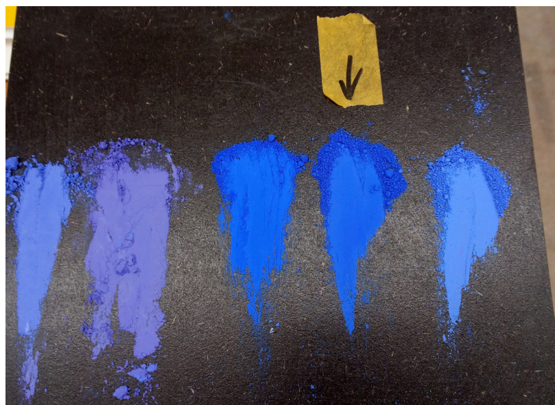
The appearance of the colour samples changes when different binders are applied
