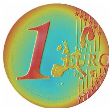
Topography of a one-euro coin measured with an optical confocal profilometer developed at the Centre for Development of Sensors (UPC). The ordinal colour scale represents the height of the surface relief. www.cd6.upc.edu
