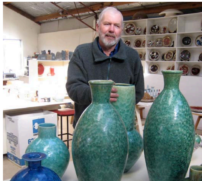
Rynne Tanton and his macrocrystal glazed ceramics have recently been featured in Vogue Living Australia. The colours are created using different metal oxides in the glaze mix – cobalt for blue, copper for green, titanium for white, etc.
