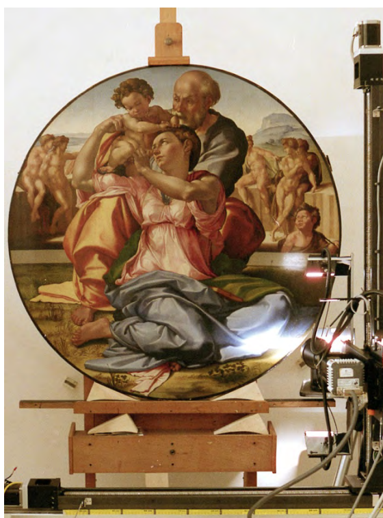
VIS-NIR hyperspectral scanner at IFAC-CNR for non-invasive reflectance measurements of art pigments.
