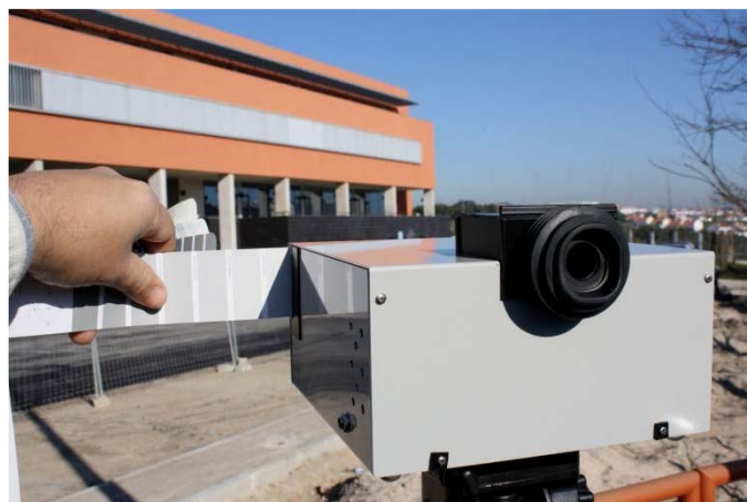
DISMECOR device and system for measuring perceived colour.
