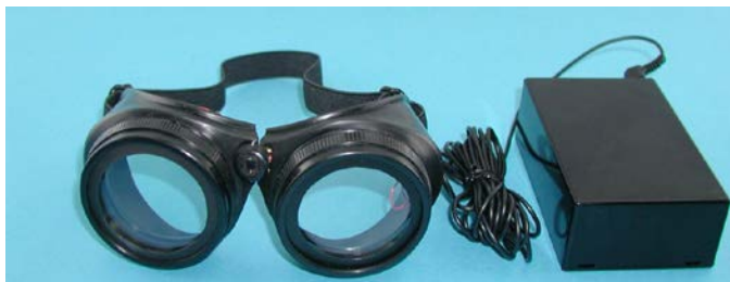
Intelligent goggles to simulate visibility in the elderly for young observers in a real environment in real time.
