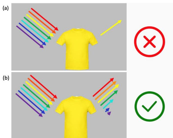
Figure 2: (a) The upper diagram illustrates the concept that a yellow object is yellow because it reflects the yellow wavelengths and absorbs the other wavelengths. It is consistent with both Axiom 1 and Axiom 2. (b) On the other hand, the lower diagram is a more realistic representation of how material reflect light.
