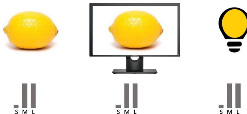
*Figure 9: A physical lemon (left), a digital reproduction of a lemon (middle), and light at wavelengths between 560 and 590nm (right) can all produce exactly the same sensation of yellow. In this case the cone responses, LMS, are identical for the three stimuli even though the wavelength distribution of the light that reaches the eye from the three stimuli may be quite different.*
