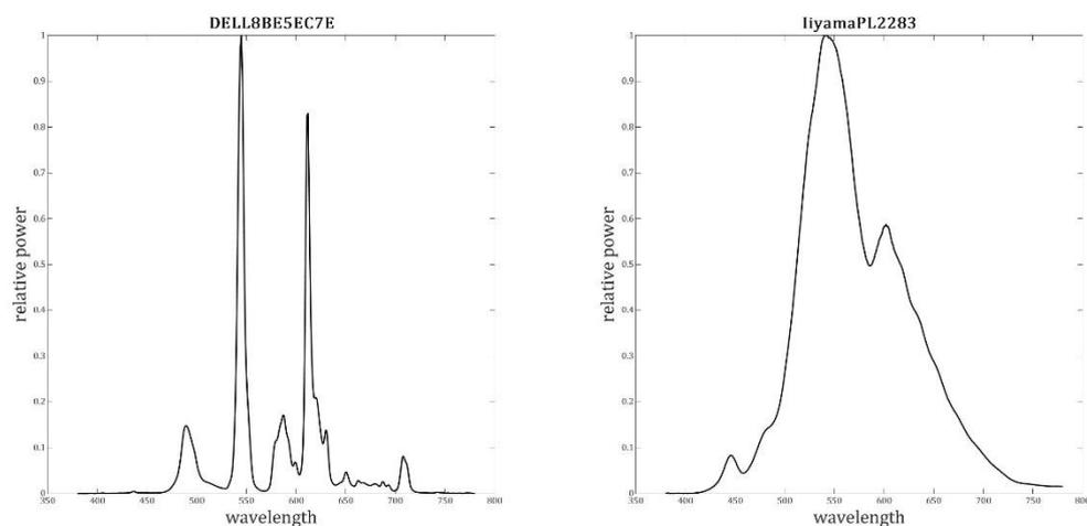
Figure 7: Spectral power measurements for two of the displays from Figure 6 when they are displaying yellow ( $R=255, G=225, B=0$ ) [33].
