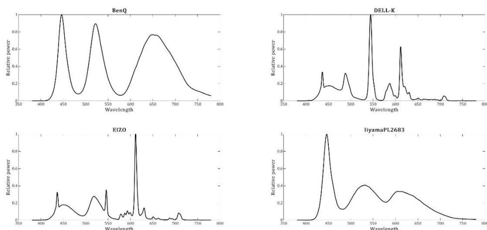
Figure 6: Measurements of the spectral power output at each wavelength when white is displayed for four different emissive displays [33]. Note that BenQ and EIZO are professional displays where the other two are consumer displays.
