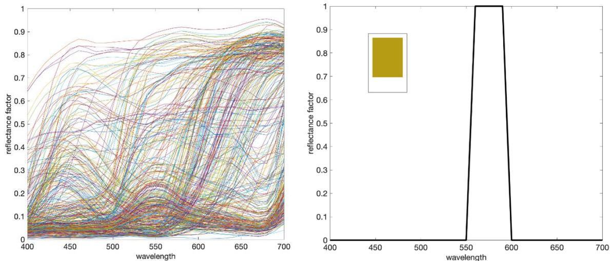
Figure 4 (left): Spectral reflectance factors for 404 different coloured samples measured from the natural world [29].
