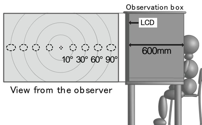
Figure 2: Experimental setup and view from the observer.
