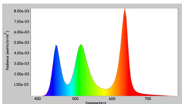
Figure 2: The spectral power distribution measured at Reference room surfaces.
