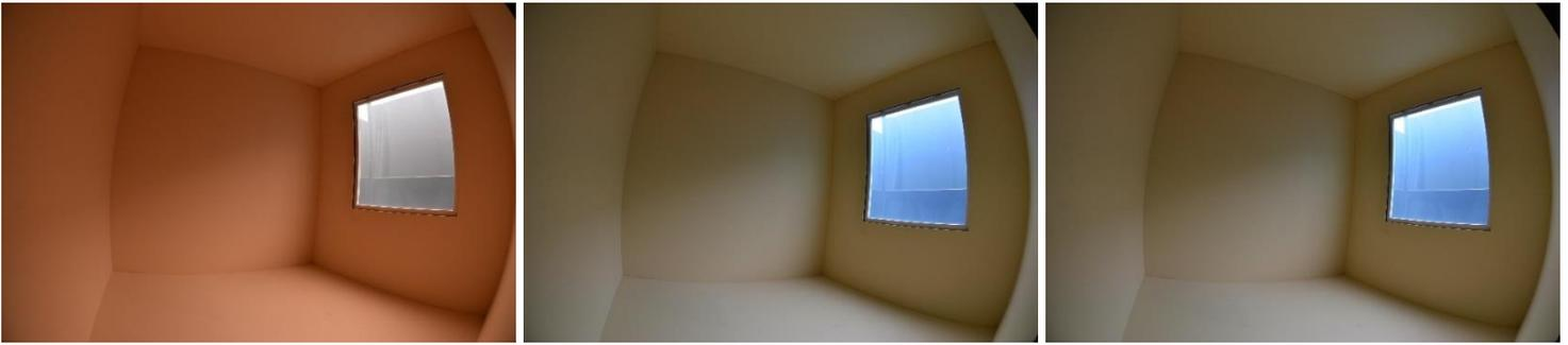
Figure 4: Box 1 (yellow box) through ET-on glazing and 2700K (left), 6500K (middle) and 8000K (right).
