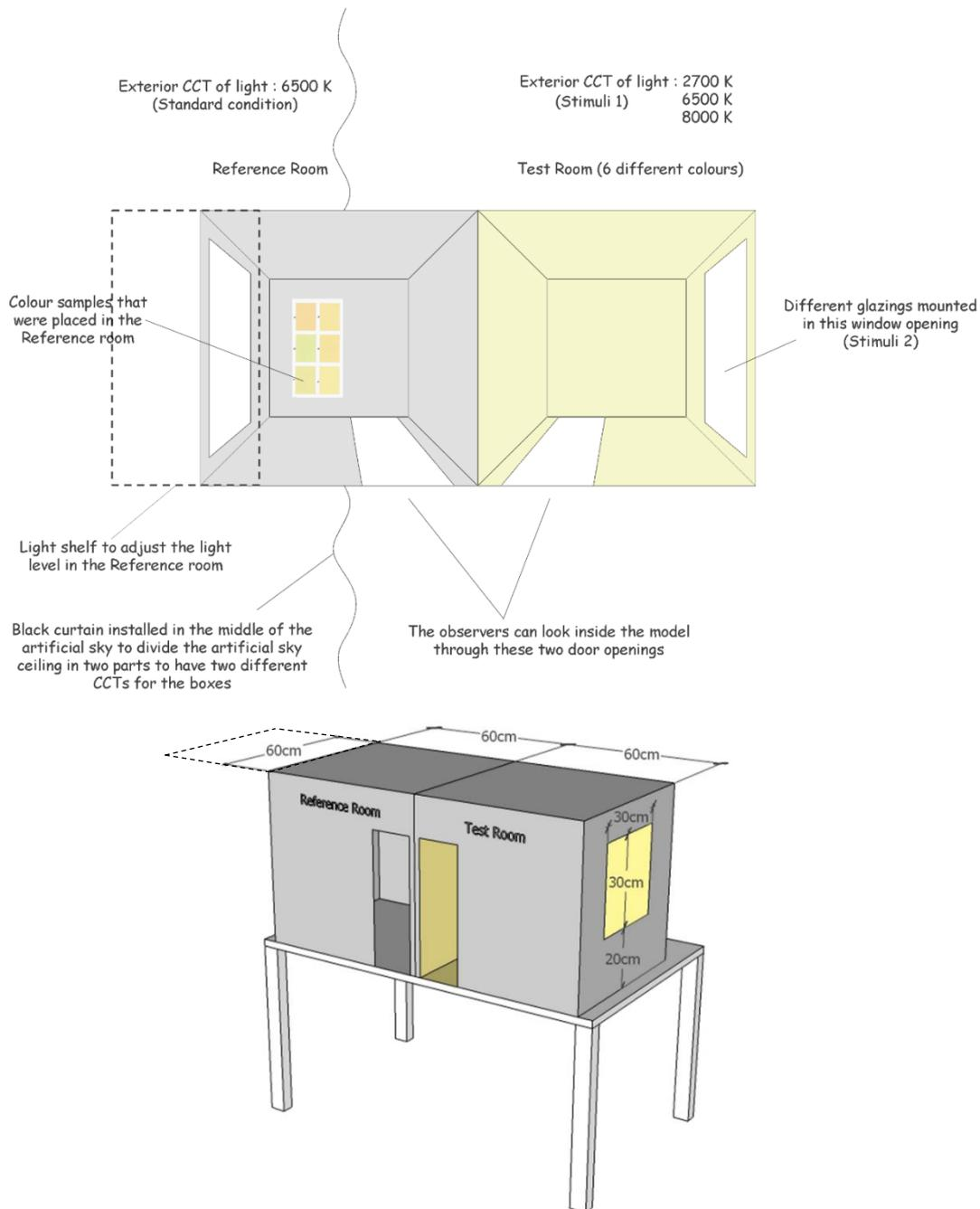
Figure 1: Experimental set-up. Above: top view, below: perspective view of the model.
