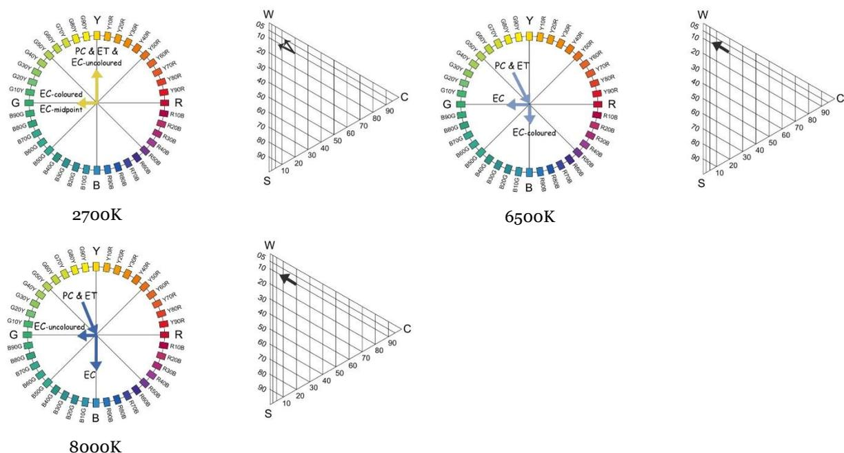
Figure 8: Colour shift tendencies for grey box at different colour temperatures.
