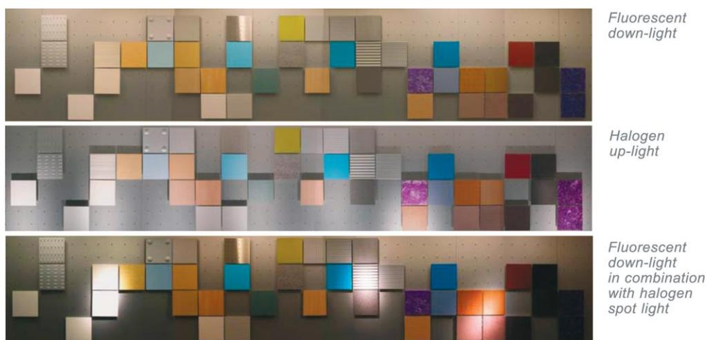
Figure 1: Material wall illuminated with fluorescent down-lights, halogen up-lights and a combination of fluorescent down-lights and halogen spots.
