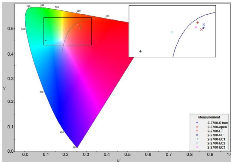
Figure 13: CIE graph for sample 2 with different glazings under 2700K.
