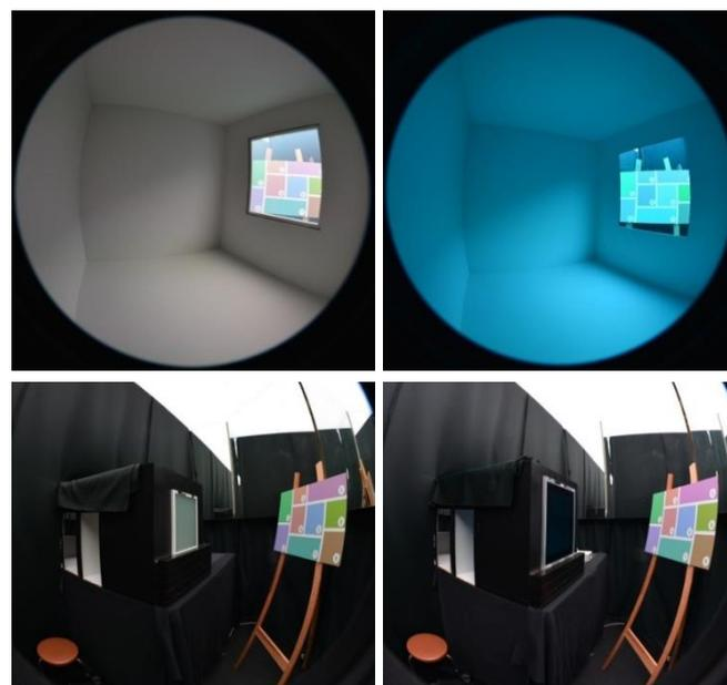
Figure 7: **Above:** Fish-eye photographs of scale models with ET glass (left) and EC-coloured glass (right).
