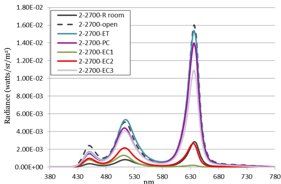
Figure 12: Comparison of spectral power distribution for sample 2 for different glazings in 2700K.
