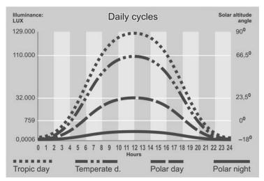
Figure 1: Around noon is the highest illumination emission and around midnight the weakest, but in correlation to solar altitude degree, the whole energy amount varies strongly with latitude.
